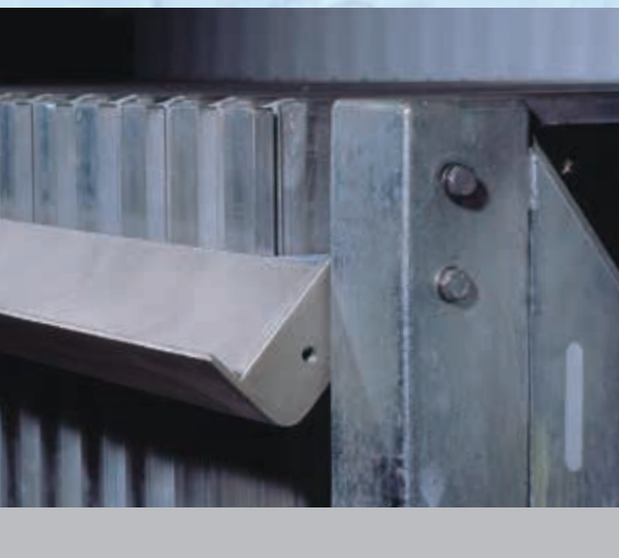
The front bar can be tipped for easy cleaning under the forks and fork linings.
