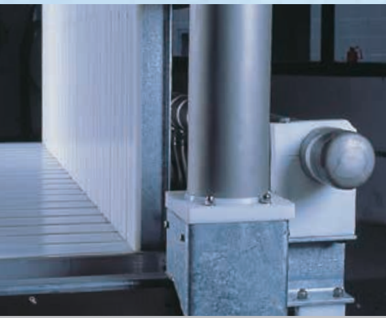
DSI Hydraulic ALU block which secures easy access and service.
